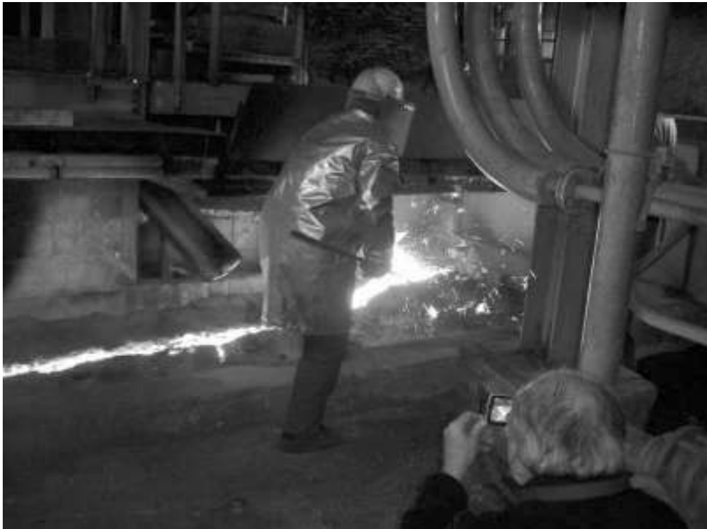
Picture 3 The first casting through the drain bottom hole
