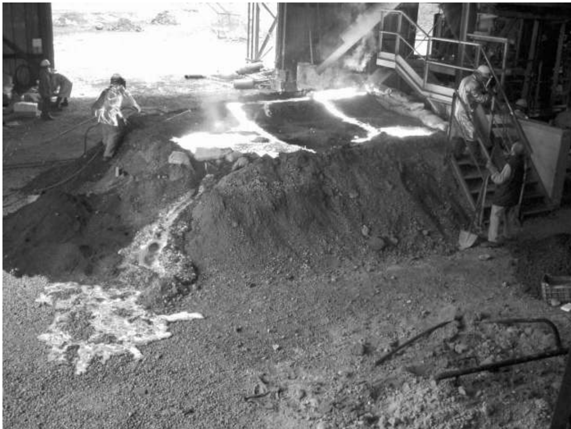
Picture 6 The first casting through the siphon
