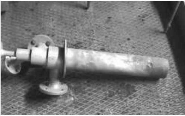
Picture 9: Failed oxy-coal lance. The failure is in the steel-copper seal area
