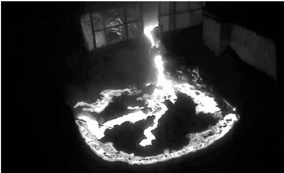
Picture 8: Hot metal tapping in a deep sand pit
