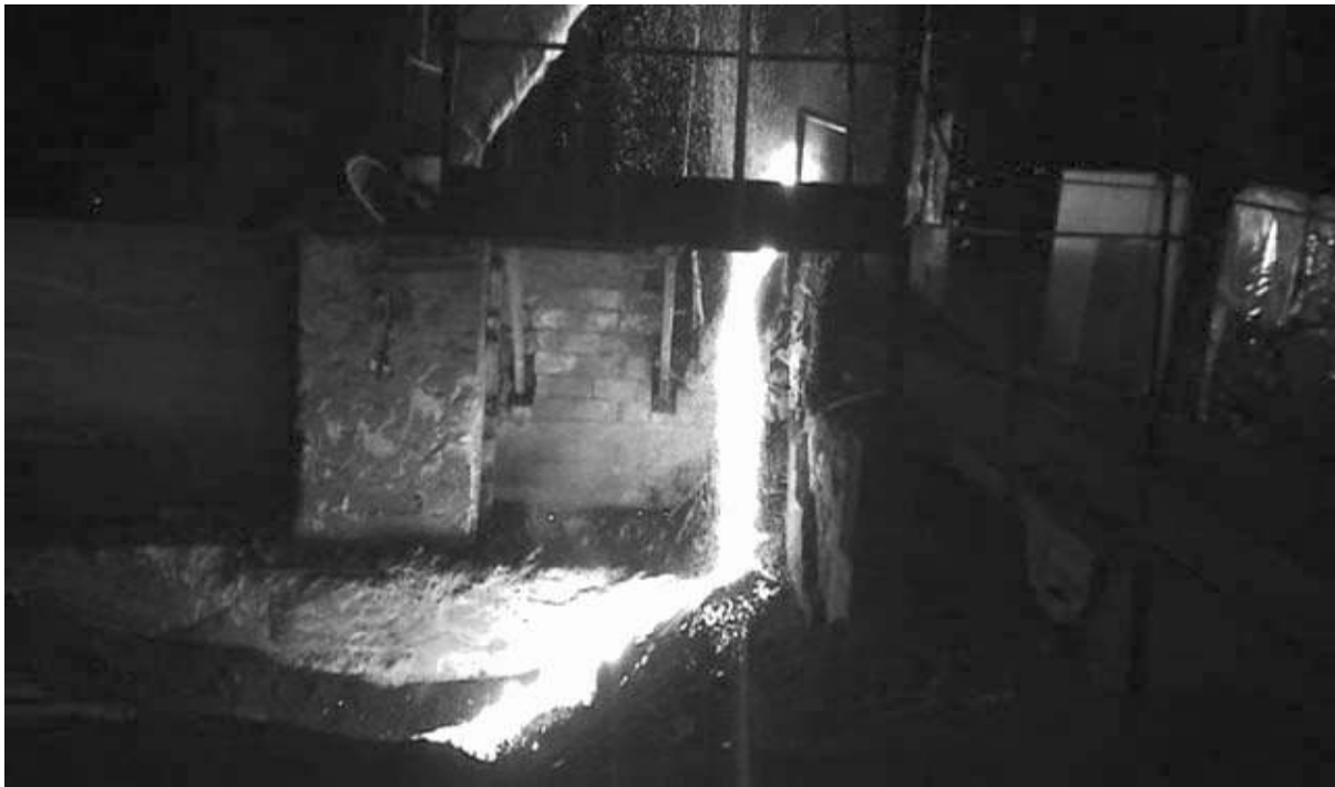
Picture 10: Continuous slag tapping from slag taphole
