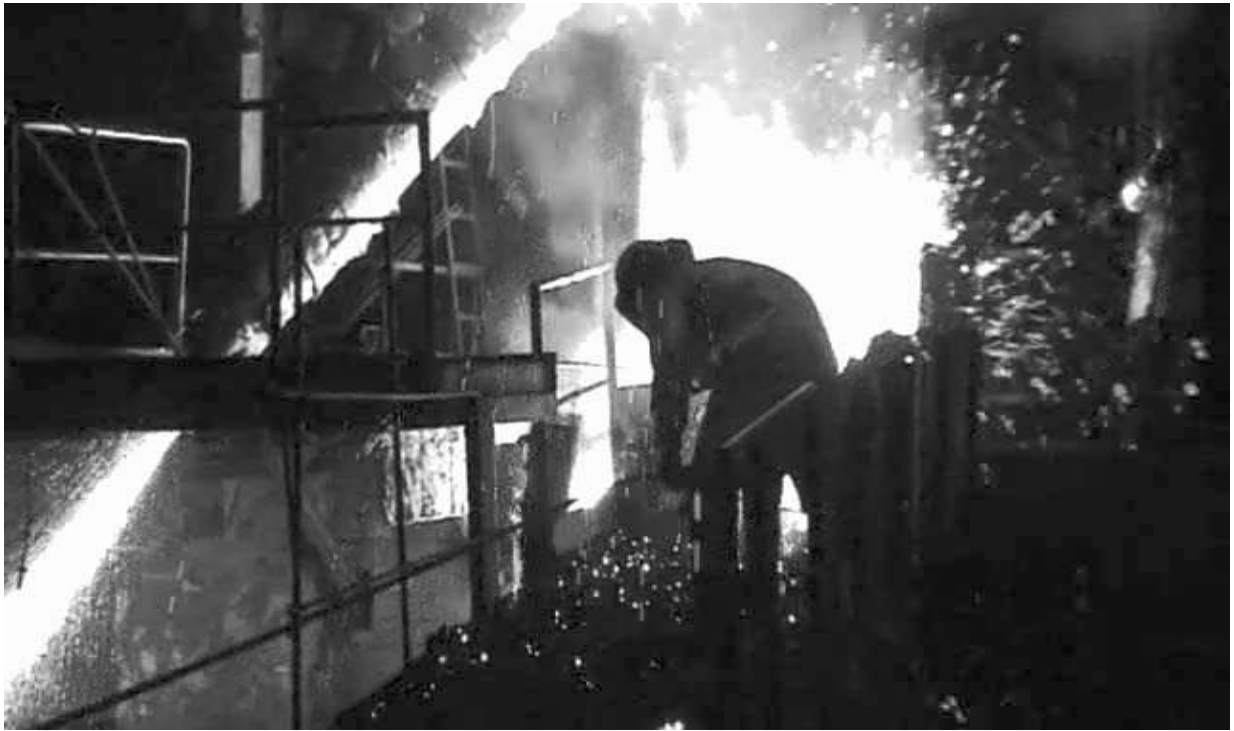
Picture 11: Opening of the hot metal taphole while hot DRI is deviated to slag pit
