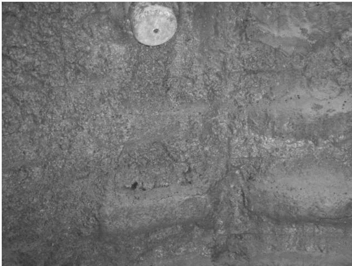
Picture 5 The slag lining formed during operation
